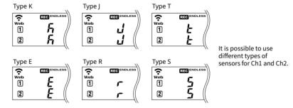
The factory default setting is "K" for both channels. Depending on the thermocouple type to be used, make settings or changes using the PC software "TR7 for Windows", mobile app "T&D Thermo", or cloud-based 'T&D WebStorage Service".
