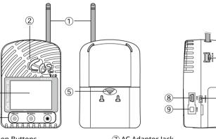
(7) AC Adaptor Jack 8) USB Connector (Mini-B) 9 Serial Connector (EXT ALM)
