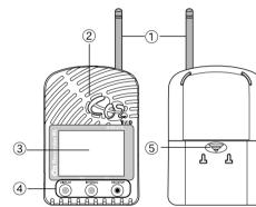
(4) Operation Buttons (DISPLAY) Button. (INTERVAL) Button (REC/STOP) Button 5) Battery Cover
