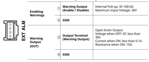
The connection between ① and ② decides whether Warning Output is enabled or disabled. If a warning condition occurs while Warning Output is enabled, a connection between ③ and ④ will be established and a warning will be output.
