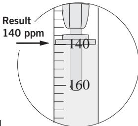
If the plunger tip reaches the bottom line on the scale (200 ppm) before the endpoint color change occurs, refill the Titrator and continue the titration.
