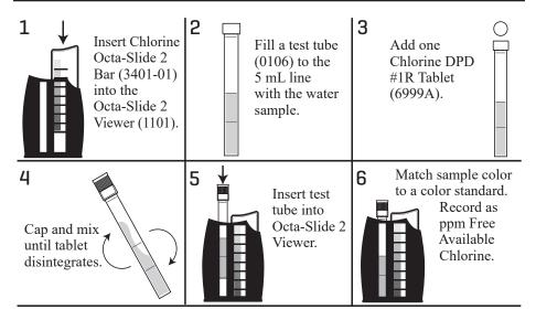
NOTE: Retain this sample if Total Residual Chlorine and Combined Chlorine are to be tested.
