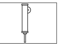
3. Use the 1.0 mL transfer pipet (2-2170) and pipette pump (30527) to add 1.0 mL of HR Reagent (3988) to each of 2 clean colorimeter tubes (0290).
