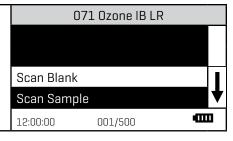
12. Insert the Reagent Blank tube into chamber, close lid and select **Scan Blank**.
