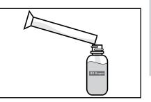
2. Use the 5 mL volumetric pipet (0329) and pipette pump (30527) to add 5 mL of Indigo Blue Stock Solution (3989) to the amber glass bottle. Cap and mix.
