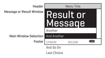
As described previously, the *EXIT* button allows an exit or escape from the current menu and a return to the previous menu. This allows a rapid exit from an inner menu to the main menu by repeatedly pushing the *EXIT* button. Pushing *C* at any time will turn the colorimeter off.
