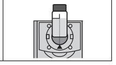
8. Press to scan the standard. The screen will display **Reading...** for about 1 second. The result will appear on the screen.
