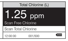
12. Subtract the Free Chlorine reading from the Total Chlorine reading to obtain the concentration of Combined Chlorine.
