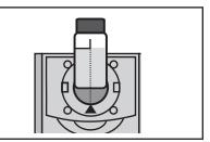
9. Press extent to select Scan Total Chlorine. The screen will display Reading... for about 1 second. The result will appear on the screen. Record the result as Total Chlorine.
