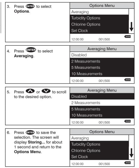
NOTE: When the **Averaging** option is enabled, more time will be required to display a reading and more power will be used.
