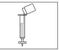
Remove the filter from the syringe. Remove the plunger from the barrel. (This step is required to prevent rupturing the filter by the vacuum that would be created when the plunger is removed.)
