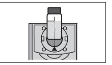
8. Press extent to scan the sample. The screen will display **Reading...** for about 1 second. The result will appear on the screen. Record the result as Free Chlorine.
