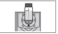
8. Press NED to scan the Standard. The screen will display **Reading...** for about 1 second. The result will appear on the screen.
