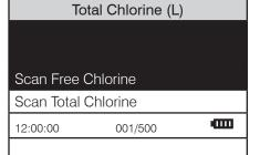
Remove the tube from the meter. Add 5 drops of DPD 1A Free Chlorine reagent (P-6740) and add 5 drops of \*DPD 1B Free Chlorine reagent (P-6741). Cap and invert to mix. The solution will be pink if chlorine is present.
