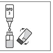
NOTE: For wastewater samples, <u>Standard Methods for the Examination of Water and Wastewater</u> recommends waiting 2 minutes for full color development when testing total chlorine.
