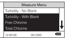
Turbidity NB (F) 3. Press ENTER to select Turbidity - No Blank. Scan Blank Scan Sample 1000 12:00:00 001/500 Rinse a clean tube (0290) three times with the sample. 5. Fill the tube to the fill line with the sample. Pour the sample down the inside of the tube to avoid creating bubbles. Cap the tube. Wipe the tube thoroughly with 6. a lint-free cloth. Open the meter lid. Insert the tube into the chamber. Align the index line on the tube with the index arrow on the meter. Close the lid.
