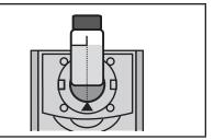
13. Press ENTED to scan the standard. The screen will display **Reading** for about 1 second. The result will appear on the screen.
