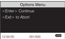
6. Press NEED to complete the Factory Reset. The screen will momentarily display Writing. The screen will display Done and return to the Options Menu. To retain the current user level calibration settings, press Net to abort the Factory Reset.
