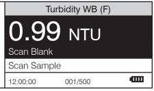
NOTE: The meter will remember the last scanned blank reading. It is not necessary to scan a blank each time the test is performed. To use the previous blank reading, instead of scanning a new one, scroll to Scan Sample and proceed. For the most accurate results, the meter should be blanked before each test and the same tube should be used for the blank and the reacted sample.
