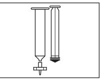
Replace the filter and repeat step 2 for a second rinse of the syringe and storage container. 5. Remove the filter from the syringe. Remove the plunger from the barrel. Replace the filter and fill the syringe with approximately 50 mL of deionized water. Filter the water into the storage container and save this turbidity-free water. 6. Repeat Step 5 until the desired amount of turbidityfree water has been collected.
