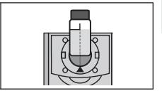
11. Press extent to select Scan Total Chlorine. The screen will display Reading... for about 1 second. The result will appear on the screen. Record the result as Total Chlorine.
