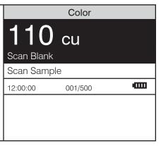
NOTE: The meter will remember the last scanned blank reading. It is not necessary to scan a blank each time the test is performed. To use the previous blank reading, instead of scanning a new one, scroll to Scan Sample and proceed. For the most accurate results, the meter should be blanked before each test and the same tube should be used for the blank and the reacted sample.
