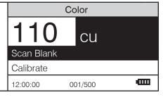
11. Press or to scroll to the concentration of the standard, 100 in this example. Note: The allowable adjustment is ±25%.
