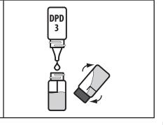
NOTE: For wastewater samples, <u>Standard Methods for the Examination of Water and Wastewater</u> recommends waiting 2 minutes for full color development when testing total chlorine.
