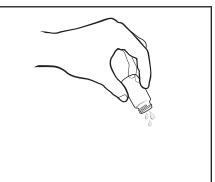
6. Fill the tube to the fill line with the blank. Pour the blank down the inside of the tube to avoid creating bubbles. Cap the tube.
