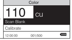
12. Press ENTED to select to Calibrate. Two menu choices will be offered, Set Calibration and Factory Settings.
