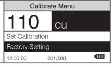
13. Press (NTE) to select Set Calibration. and save the calibration. Press or to scroll to and select Factory Setting to revert to the factory calibration. The meter will momentarily display Storing... and return to the Color menu. The calibration has now been saved and the meter can be used for testing.
