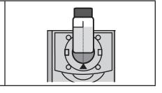
8. Press Test to scan the sample. The screen will display **Reading...** for about 1 second. The result will appear on the screen. Record the result as Free Chlorine.
