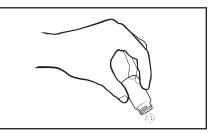
11. Fill the tube to the fill line with the standard. Pour the standard down the inside of the tube to avoid creating bubbles. Cap the tube.
