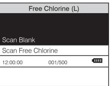
Remove the tube from the meter. Add 5 drops of DPD 1A Free Chlorine reagent (P-6740) and add 5 drops of \*DPD 1B Free Chlorine reagent (P-6741). Cap and invert to mix. The solution will be pink if chlorine is present. Read within 30 seconds.
